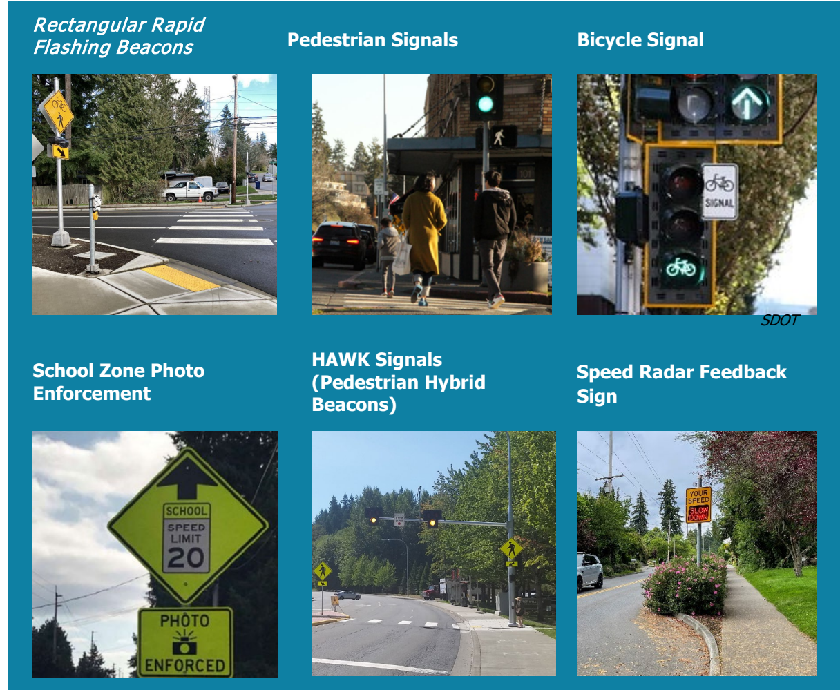
FIGURE 3-22 EXAMPLES OF TRAFFIC CONTROL DEVICES IN KIRKLAND
