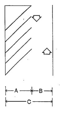
\*For a double loaded aiste containing standards size stalls on one side and compact size stalls on the other side, the required driving aisle width (Column E) shall be the required width for standard size stalls.
