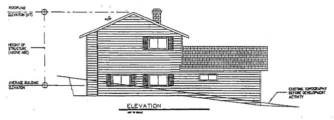
NOTE: PLEASE INCLUDE THE ELEVATION OF THE RIDGE OF THE ROOF ROOFLINE ON THE SITE PLAN AND/OR INDICATE ON THE ELEVATION DRAWINGS WHERE THE AVERAGE BUILDING ELEVATION (CALCULATED ABOVE) STRIKES THE BUILDING.
