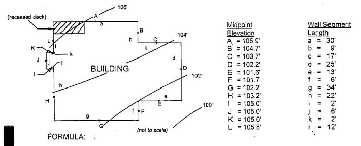
$\frac{(A \times a) + (B \times b) + (C \times c) + (D \times d) + (E \times e) + (F \times f) \dots + (L \times I)}{a + b + c + d + e + f \dots + I} = \text{Average Building Elevation (ABE)}$
