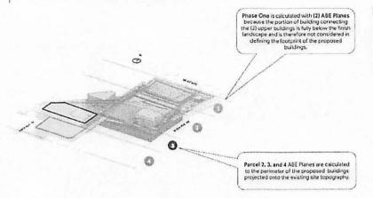
The plan extents of the "Average Building Elevation" for zoning shall be traced around the perimeter of portions of buildings with wells 4 or taller above finished grade. These footprints are projected onto the existing site topography to determine the ABE for each building. The Northern Mid-Block Connection is at grade, so there will be two ABE calculations for the Phase I structure.
