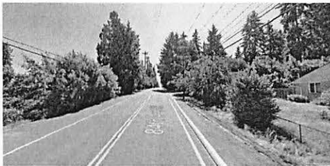
Example of a curb protected shoulder on 84th Ave NE in Kirkland, Washington
