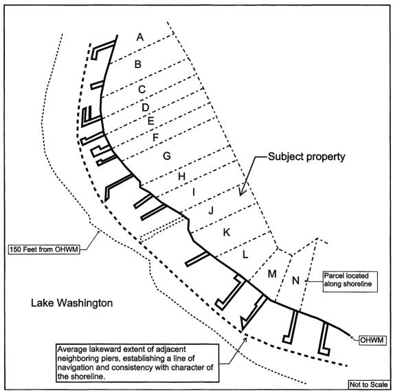
Parcel 'J' needs to establish the allowable length a pier may extend under the development regulations of section 83.270. Since the 150 foot measurement from the OHWM exceeds the average lakeward extent of the adjacent neighboring piers, the lesser applies. Parcel 'J' may propose a pier length as shown, aligning with the average lakeward extent of the adjacent neighboring piers. The pier is subject to all other dimensional standards, including but not limited to width, area, and height.
