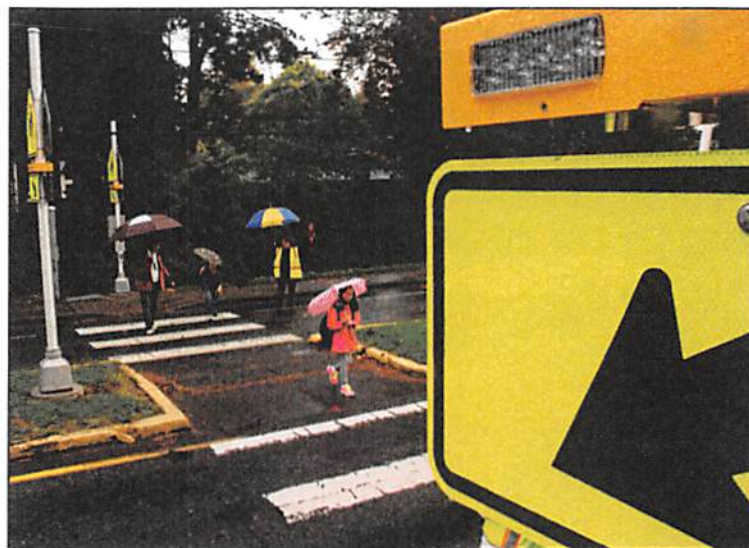
An elementary school student uses Rapid Flashing Beacons on Northeast 116th Street.
