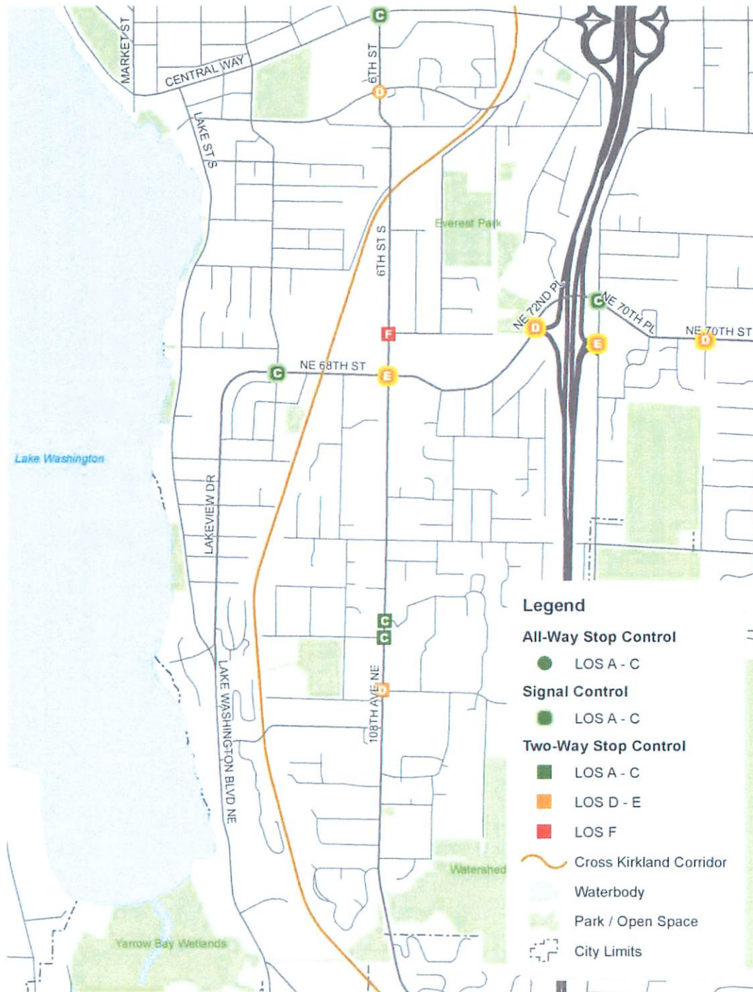
Figure 10 - PM Peak Intersection Level of Service
