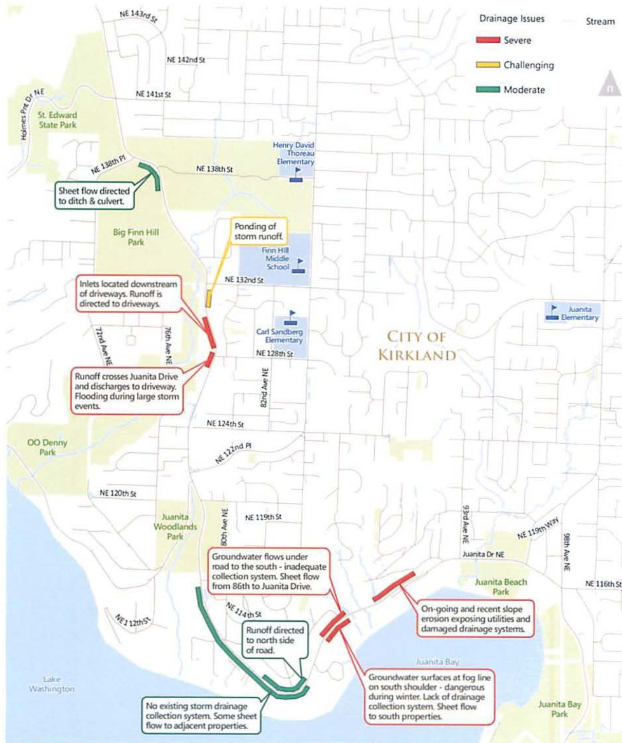
FIGURE 6: DRAINING ISSUES AND CONCERNS
