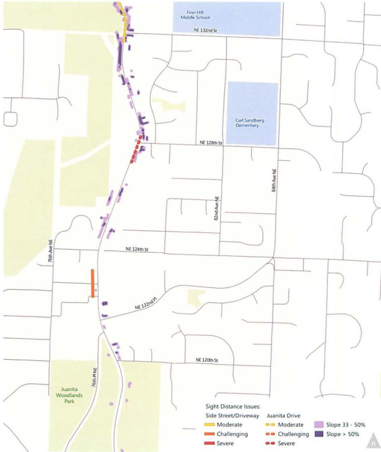
FIGURE 5B: SLOPE AND SIGHT DISTANCE – CENTRAL
